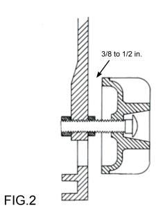
Bolt the Automatic Draft Control through the 1/2 in. hole in the center of the bottom door. Be sure to hold the Draft Control straight while tightening. Feed the two wires from the draft motor through the flexible conduit and a 90° fitting. Secure the fitting to the draft motor and that end of the conduit at this time. Check the flapper door on the Automatic Draft Control assuring that it moves freely.
